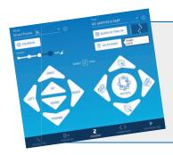
Smart Frame's patented technology determines the user's orientation relative to the robot. This eliminates the use of conventional coordinate (X, Y, Z) frames and utilizes intuitive natural language directions for easy command of the robot movement.
