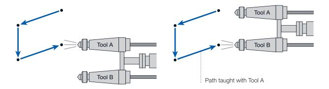
After teaching with Tool A, apply undercoat using Tool A. 2. With this function, apply top coat using Tool B.
